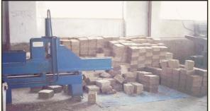
• A Complete Feed Block making machine was developed, tested and used for making CFBs for different categories of goats.
