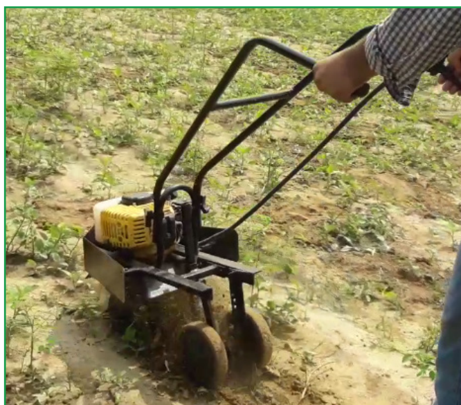
Fig.4 Developed power weeder operating in the crop field
