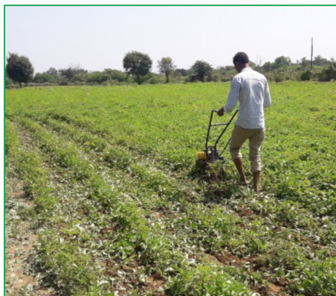
Fig.4 Developed power weeder operating in the crop field
